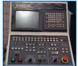
HANKOOK VTC-140E , Fanuc 21i-TB Control, Live Tool, C Axis, Chuck Size 55", Max Swing 63", Turning Height 55", Travels: X-63", Z-35.4", 24 ATC, 50 Taper, 12 Live, 12 Turning, Ram Size 8.66" Square, Rapid Traverse Rates X&Z- 472 IPM, Max Chuck Speed 320 RPM, Milling Spindle Speed 30-3,000 RPM, Main Motor 60 HP, Milling Spindle Motor 25 HP, Chip Conveyor, sn 39C08467
