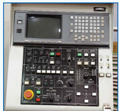
YOUJI Model YV-2000 ATC+C , Fanuc 18TL Control, Live Tool, C Axis, Chuck Size 79", 4 Jaw, Max Swing 98", Max Cutting Height 63", Max Cutting Diameter 91", Travels: X-73", Z-39", Vertical Travel of Crossrail 45", 16 ATC, 50 Taper, Table Speed Low 2-50 RPM, High 50 -200 RPM, Rapid Traverse of Railhead X&Y Axes - 394 IPM, Cutting Feed Rate 500 IPM, Spindle Motor 100 HP, Max. Tool Weight 110 lb, Max Table Load 22,000 lbs, Chip Conveyor, Machine Weight 101,200 lb, sn 01V20T0469
