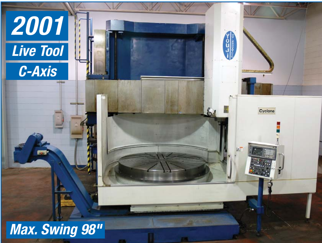
YOUJI Model YV-2000 ATC+C , Fanuc 18TL Control, Live Tool, C Axis, Chuck Size 79", 4 Jaw, Max Swing 98", Max Cutting Height 63", Max Cutting Diameter 91", Travels: X-73", Z-39", Vertical Travel of Crossrail 45", 16 ATC, 50 Taper, Table Speed Low 2-50 RPM, High 50 -200 RPM, Rapid Traverse of Railhead X&Y Axes - 394 IPM, Cutting Feed Rate 500 IPM, Spindle Motor 100 HP, Max. Tool Weight 110 lb, Max Table Load 22,000 lbs, Chip Conveyor, Machine Weight 101,200 lb, sn 01V20T0469
