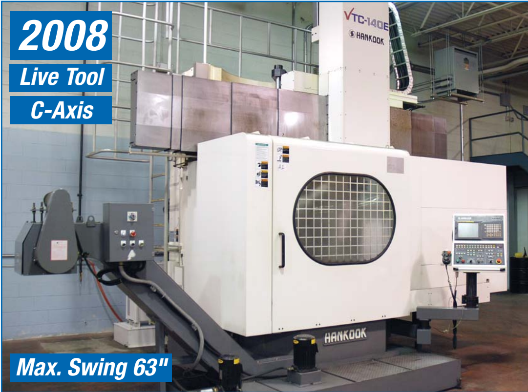
HANKOOK VTC-140E , Fanuc 21i-TB Control, Live Tool, C Axis, Chuck Size 55", Max Swing 63", Turning Height 55", Travels: X-63", Z-35.4", 24 ATC, 50 Taper, 12 Live, 12 Turning, Ram Size 8.66" Square, Rapid Traverse Rates X&Z- 472 IPM, Max Chuck Speed 320 RPM, Milling Spindle Speed 30-3,000 RPM, Main Motor 60 HP, Milling Spindle Motor 25 HP, Chip Conveyor, sn 39C08467
